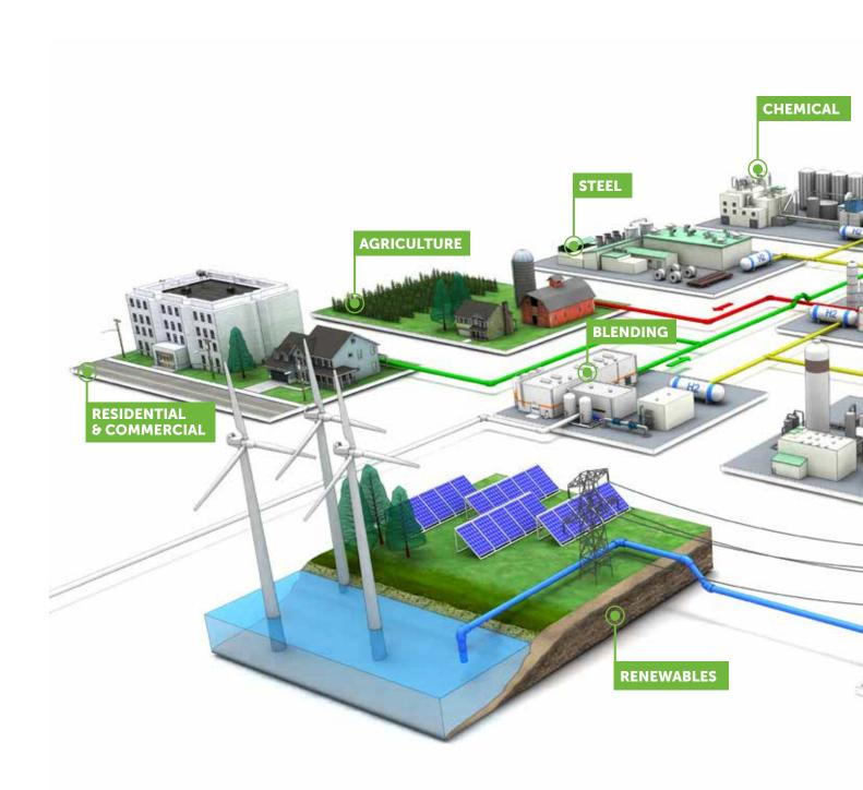
**Power-to-X** describes the process of converting renewable energy into hydrogen via water electrolysis. The produced green hydrogen can then be used as a fuel or feedstock in a variety of applications, many of which renewables alone have a hard time penetrating. Green hydrogen acts as the bridge between renewables (Power) and a multitude of downstream sectors (X).
