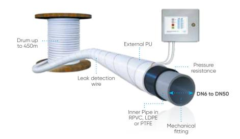
In the event of a leak, the fluid enters the interstitial space and causes a short circuit between copper wires. By connecting these wires to the system of dosage and distribution, it is possible to immediately interrupt circulation to prevent any risk of contamination and exposure.
