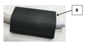
Insert the hose into the heat shrink tube (B), ensuring it covers the end of the resistor and all exposed sensor wire.
