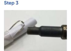
Heat the sleeves until they have shrunk completely and the solder rings have melted and flowed. Keep the heat source moving to avoid charring. Do not move the joint until it has cooled as this may weaken the joint.
