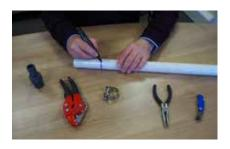
Mark a ring around the hose approximately at a point which is 2 to 2 ½ times the depth of the fitting. Mark 4 points around the hose where you will score it.
