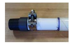
Slide on the stainless steel band clamp, then insert the fitting and tighten the clamp.
