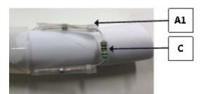
Insert the 82k  $\Omega$ resistor (C) into the ends of the solder sleeves ensuring the ring of solder is in contact with all of the wires.
