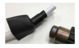
Heat until the heat shrink tube has fully shrunk and is smooth. Keep the heat source moving to avoid charring.
