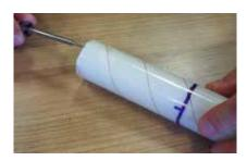
Using a small screwdriver, ease up the end of the outer PU cover.
