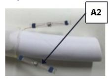
Slide a large solder sleeve (A2) on to each exposed length of wire. Cut away 50 mm of the black outer sleeve on the leader cable and trim 10mm to expose the strands (D).
