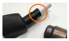
Inspect the exposed adhesive where the hose and tube join. This small bead of exposed adhesive creates the seal. Allow to cool completely.
