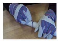
Using a sharp box cutter score the outer PU cover approximately 0.5mm deep (you want to avoid damaging the inner hose). 10mm from the end of the hose, go right the way through. Repeat this at each mark.
