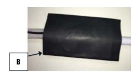
Insert the hose into the heat shrink tube (B), ensuring it covers the end of the resistor and all exposed sensor wire.
