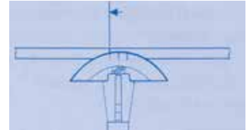
2 - Place pipe in bending tool
