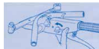
4 - Release the ratchet to free the pipe
