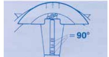
2 - Place pipe in bending tool
